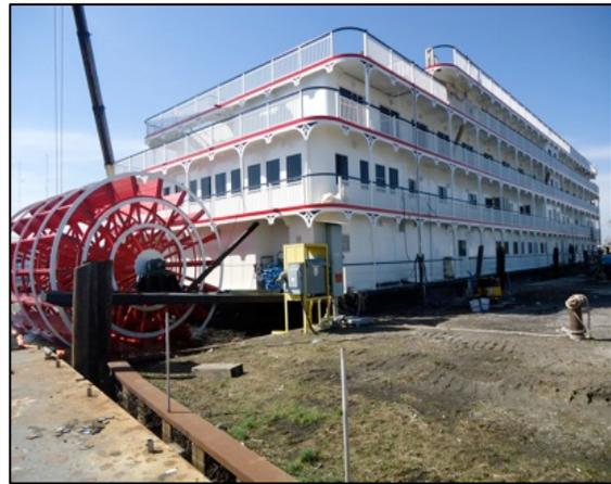
A Mascoat Specialist determined that 100 mils of Mascoat Sound Control-dB would be the ideal solution to keep the vessel quiet and the passengers happy. Chesapeake Shipbuilding sprayed the coating on decks, bulkheads and some pipes to help stop the transfer of the noise.
