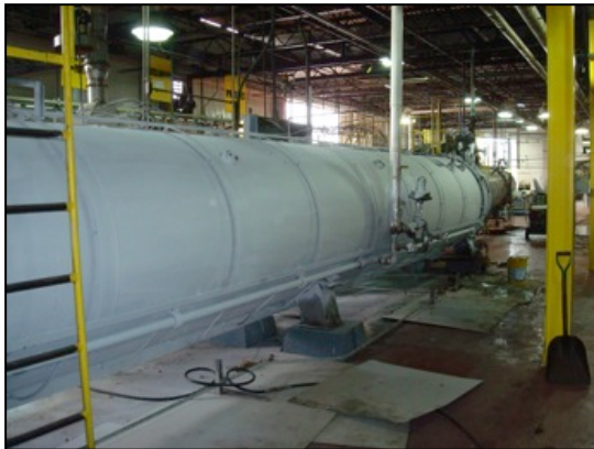
Figure 4 - Cookers after being coated with Mascoat Industrial-DTI
