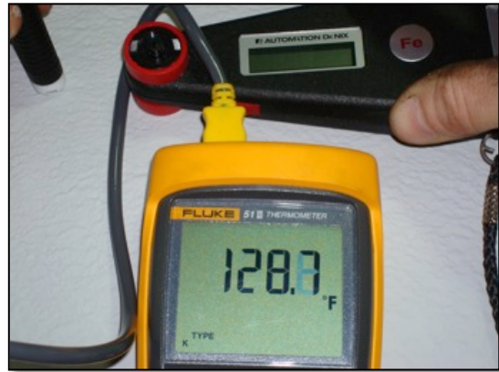
Figure 5 - Probe thermometer showing surface temperature of 128.7°F at 140 mils
